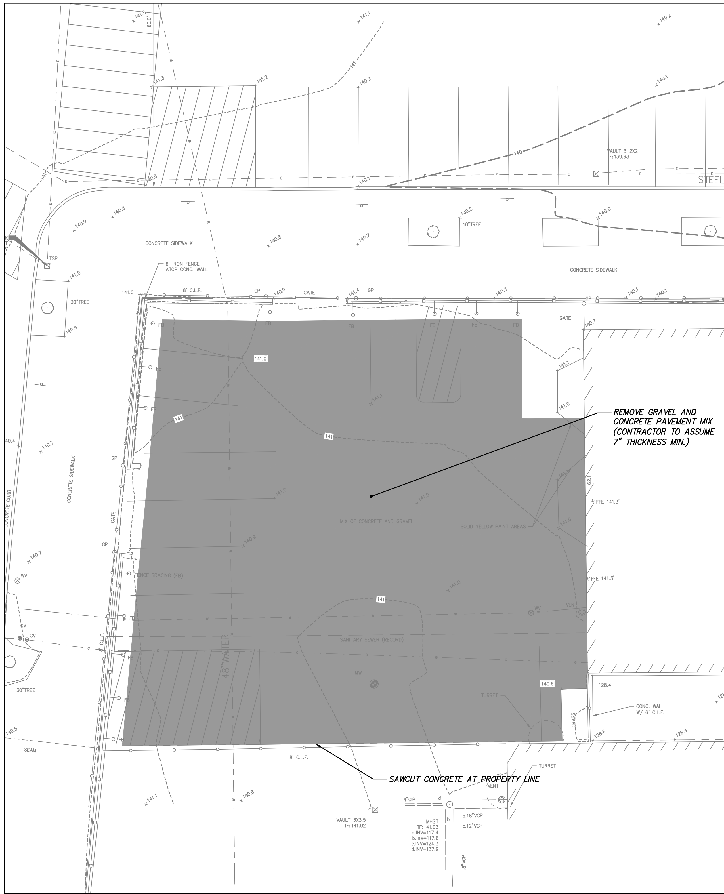
1 ALTERNATE 1: DEMOLITION PLAN SCALE: 1" = 10'
